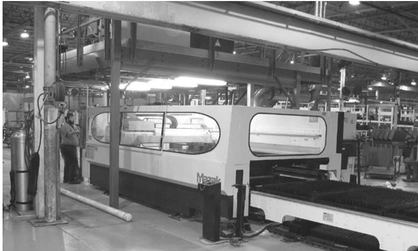
Vermeer's new ultra high performance, laser-processing machine
