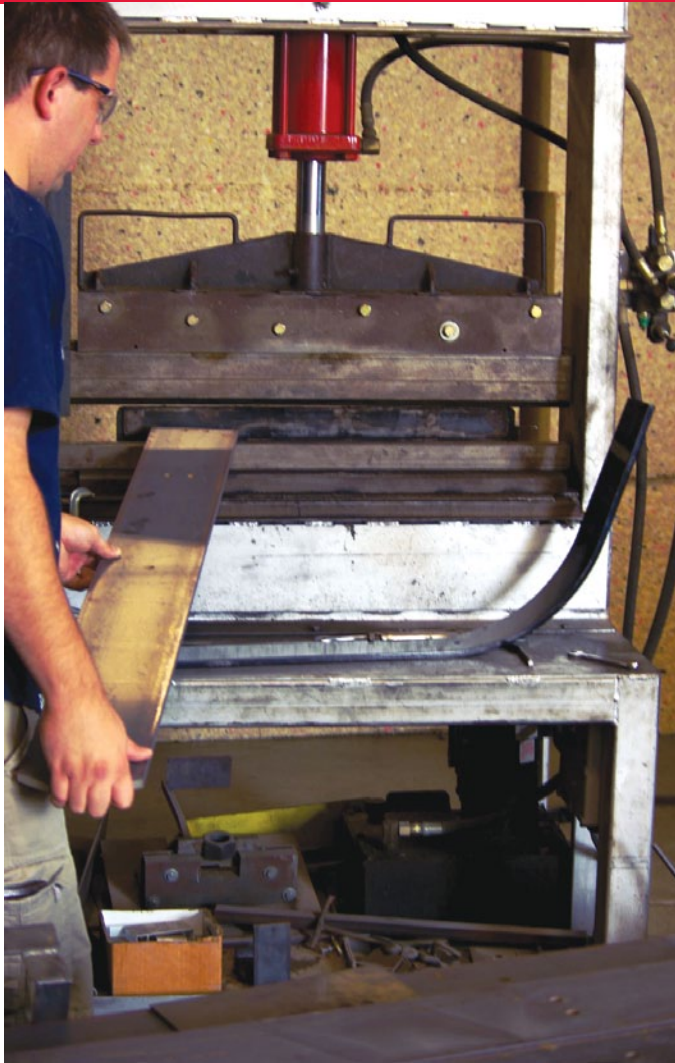
At Hadar Athletic, Jon Christensen places a flat L-bar blank into the press.
