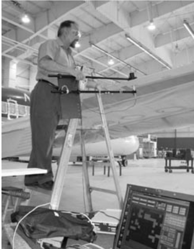
Vinay Dayal conducts nondestructive testing of an aircraft’s composite panel.
