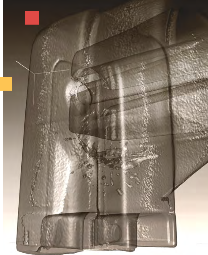
Putco product casting showing internal void.
