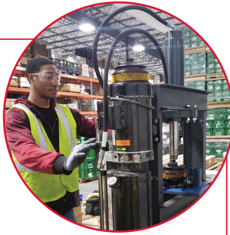
A World Class Industries employee press fits parts together for a custom order.
